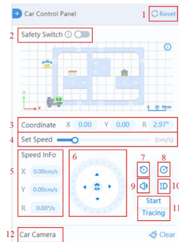
Figure 4.24 Car control panel
